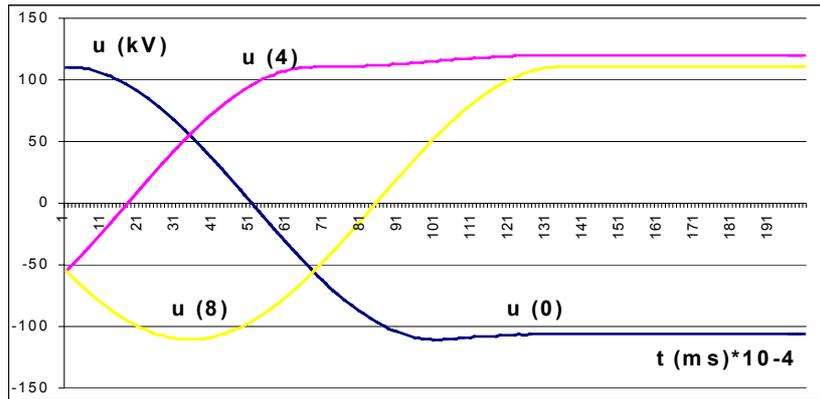
Figure 4. Transient phase to neutral voltages  $u_0$ ,  $u_4$  and  $u_8$  on the end of overhead line Podgorica1 - Bar in the case of switching off in TS Bar
