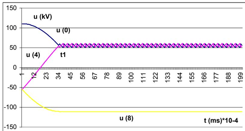
Figure 3. Transient phase to neutral voltages  $u_0$ ,  $u_4$  and  $u_8$  on the end of overhead line Podgorica1 - Bar in the case of line energizing in TS Bar
