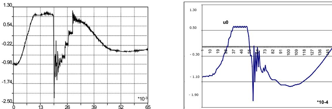
Figure 7. Transient phase to neutral voltage on the end of unloaded overhead line Podgorica1 - Budva
