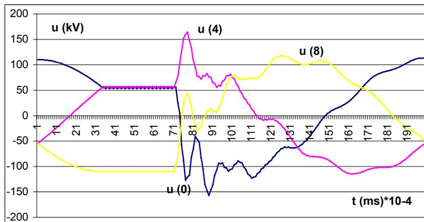
Figure 5. Transient phase to neutral voltages  $u_0$ ,  $u_4$  and  $u_8$  on the end of overhead line Podgorica1 - Budva in the case of line energizing in TS Budva by taking into consideration re-ignition of electric arc
