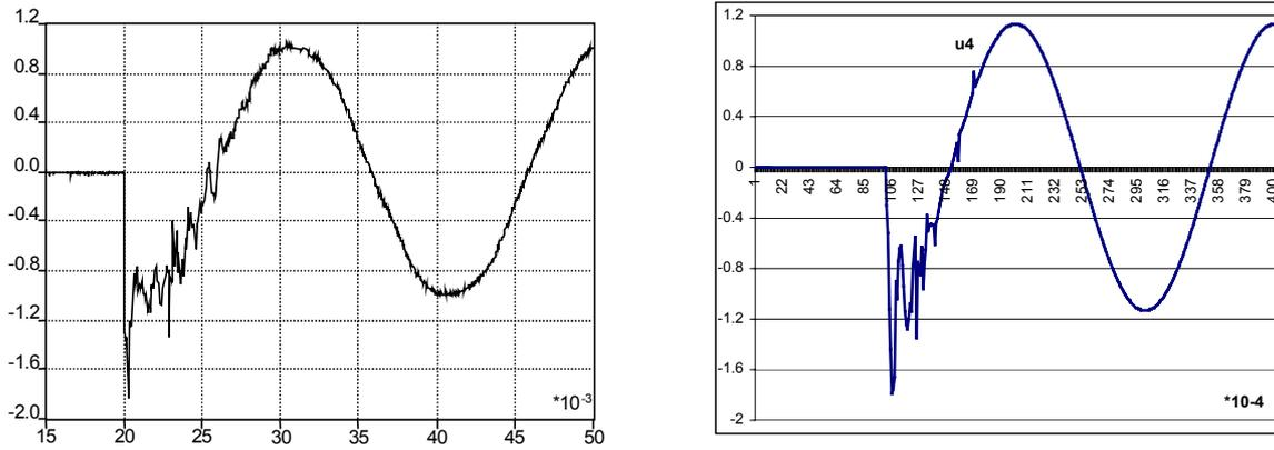
Figure 6. Transient phase to neutral voltage on the end of unloaded overhead line Podgorica1 - Budva
