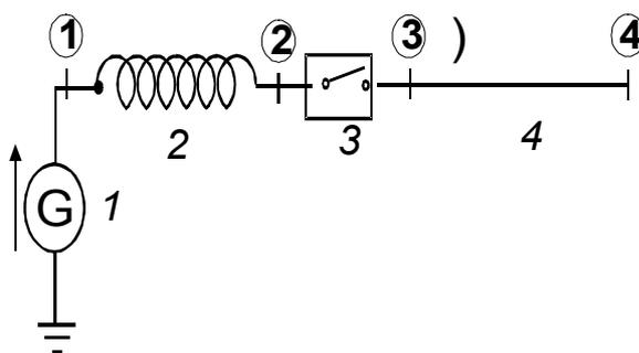
Figure 1. Model for calculation of switching overvoltages
