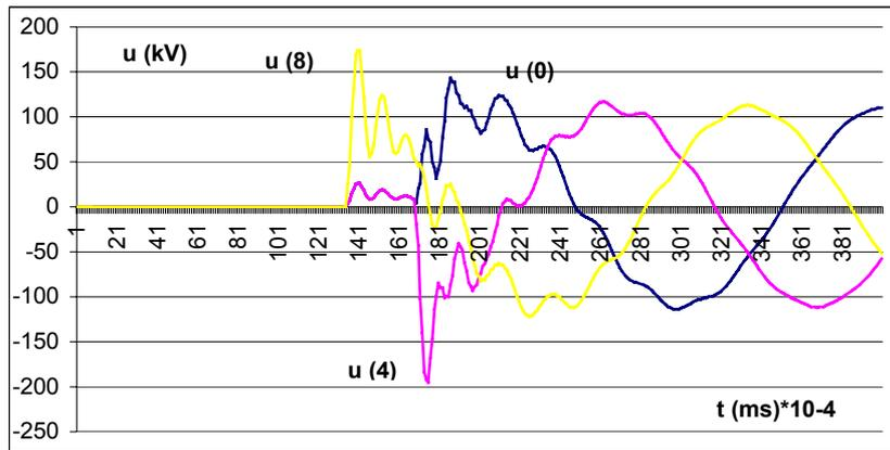
Figure 2. Transient phase to neutral voltages  $u_0$ ,  $u_4$  and  $u_8$  on the end of overhead line Podgorica1 - Budva in the case of line energizing in TS Budva
