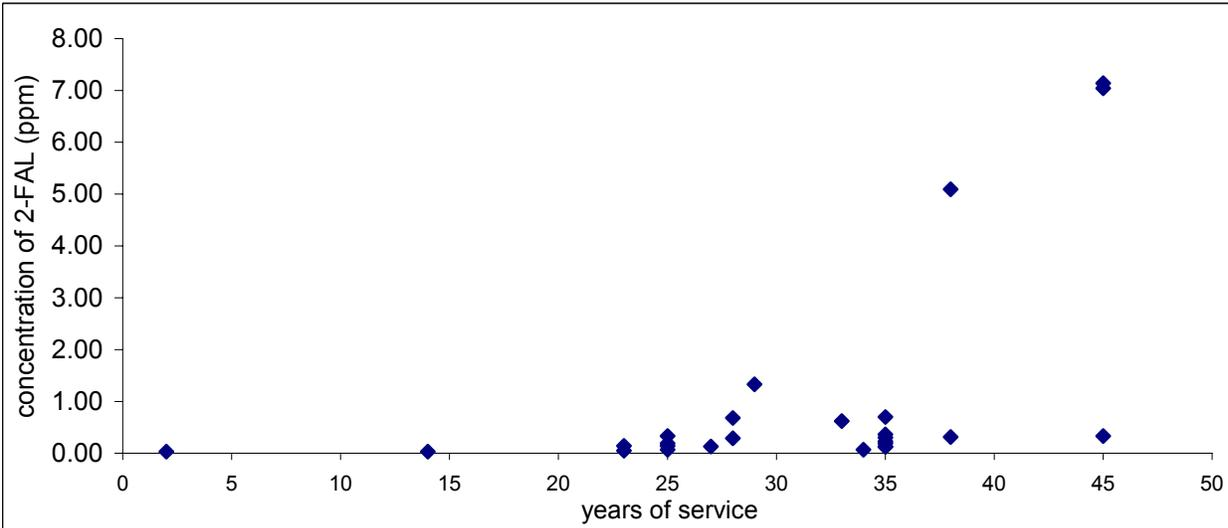
Figure 8. Correlation of 2-FAL content with years of service in 110 kV distribution network
