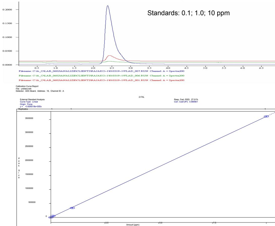
Figure 4. Chromatogram of standard solution of 2-FAL in oil and calibration curve
