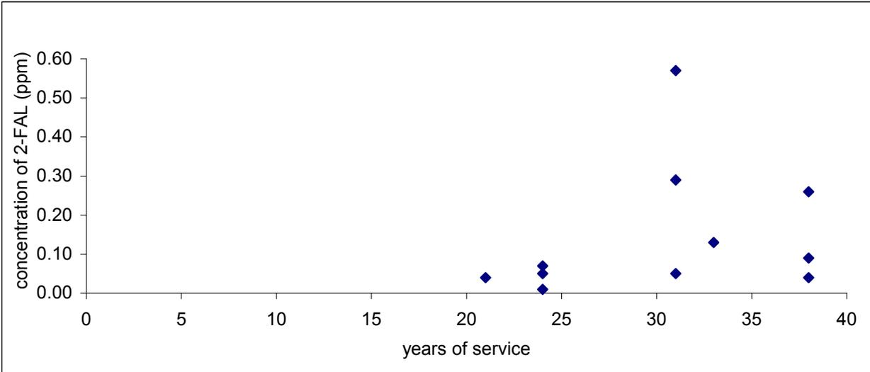
Figure 7. Correlation of 2-FAL content with years of service in hydro-power plant
