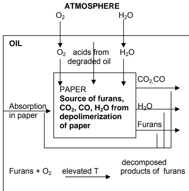
Figure 3. Scheme of simultaneous processes of furans distribution in dual paper-oil system in communication with surroundings
