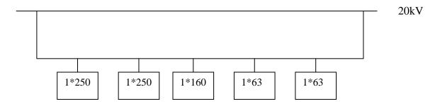
The transformers will be connected by derivation to the medium voltage network. Low voltage supply will be accomplished from the transformers low voltage panel.
