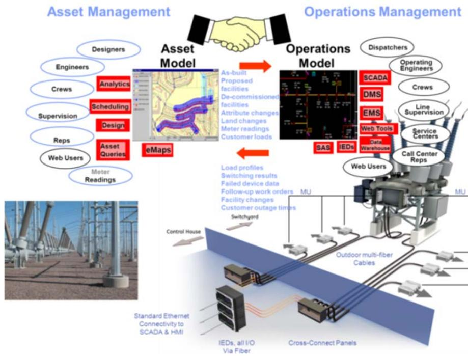
Figure 4: Vision of the Smart Substation
