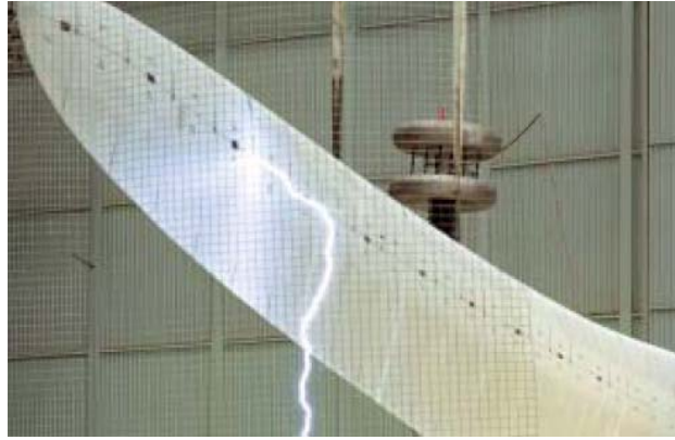
Figure 5: Wind turbine blade lightning impulse voltage test
