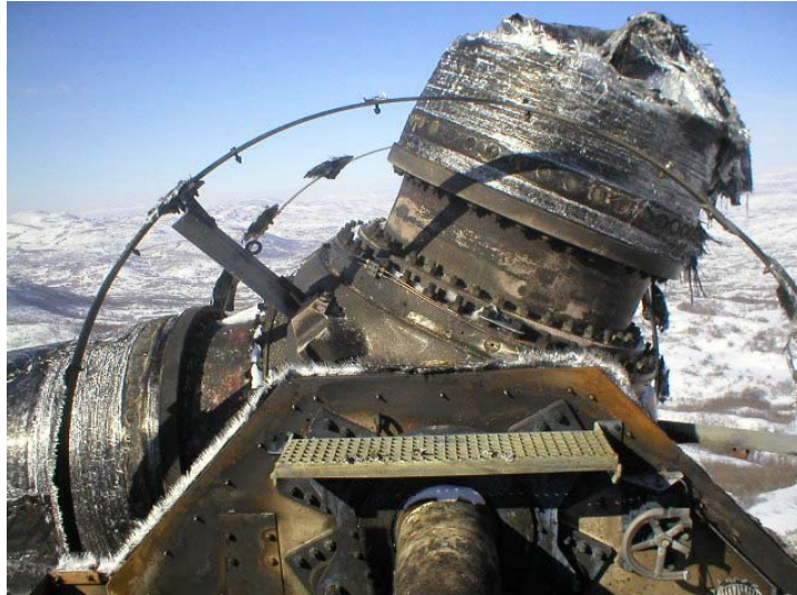
Figure 8: Destroyed wind turbine hub
