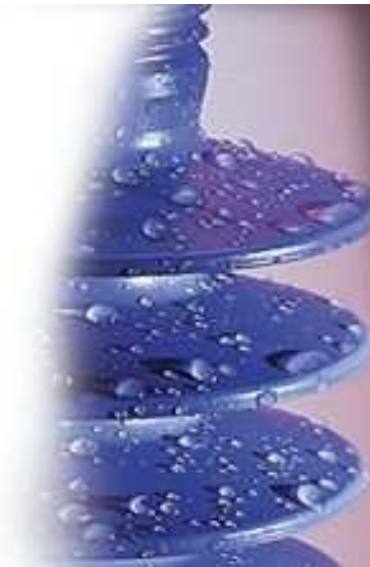
Figure 1: Water drops on the surface of silicon layered insulator
