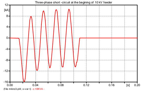
Fig. 2 Three-phase short-circuit current at the beginning of 10 kV line
